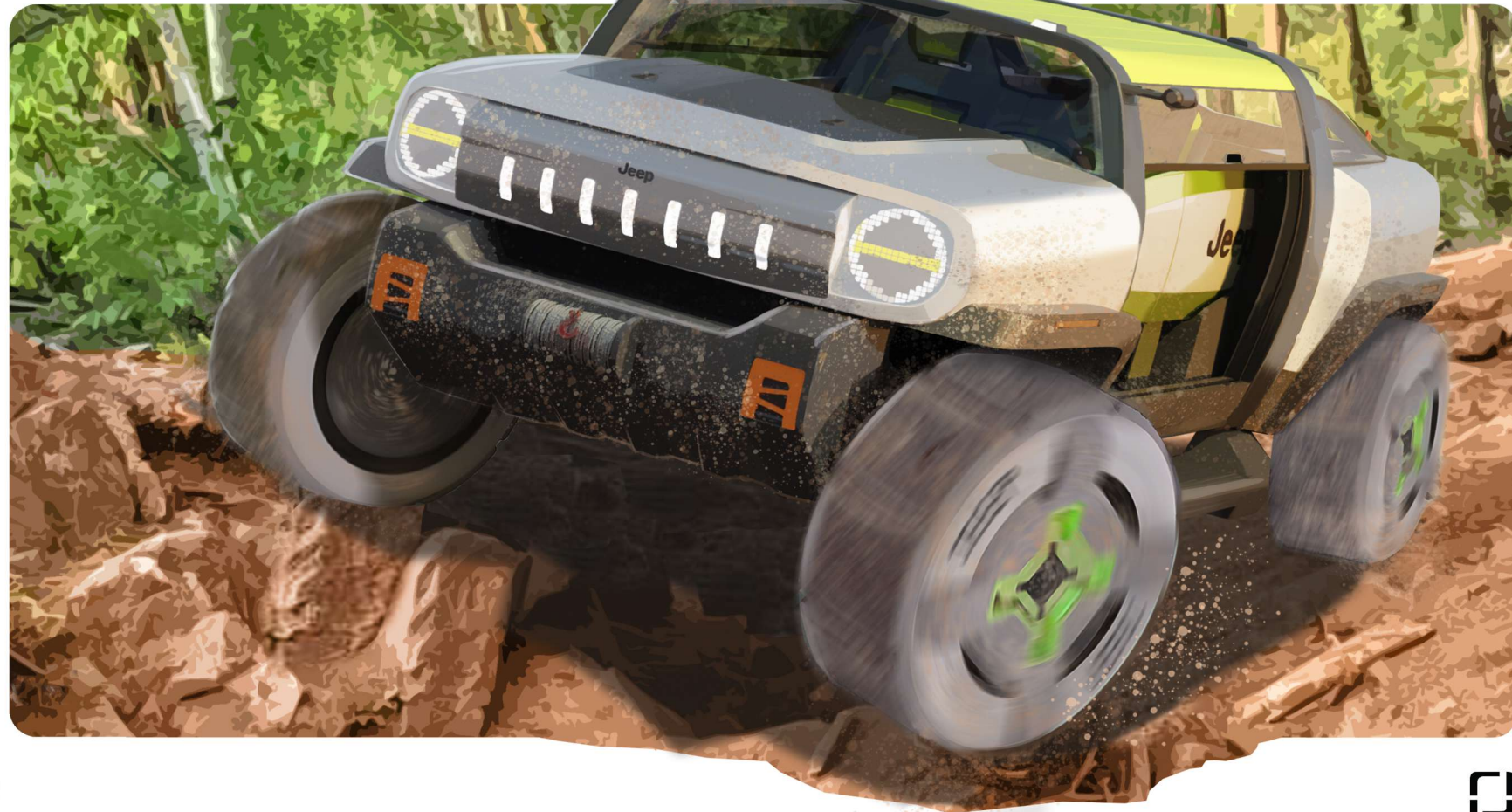
2. Driving Mode Surfboards are mounted on both sides of the vehicle and become integrated into the body when driving.
