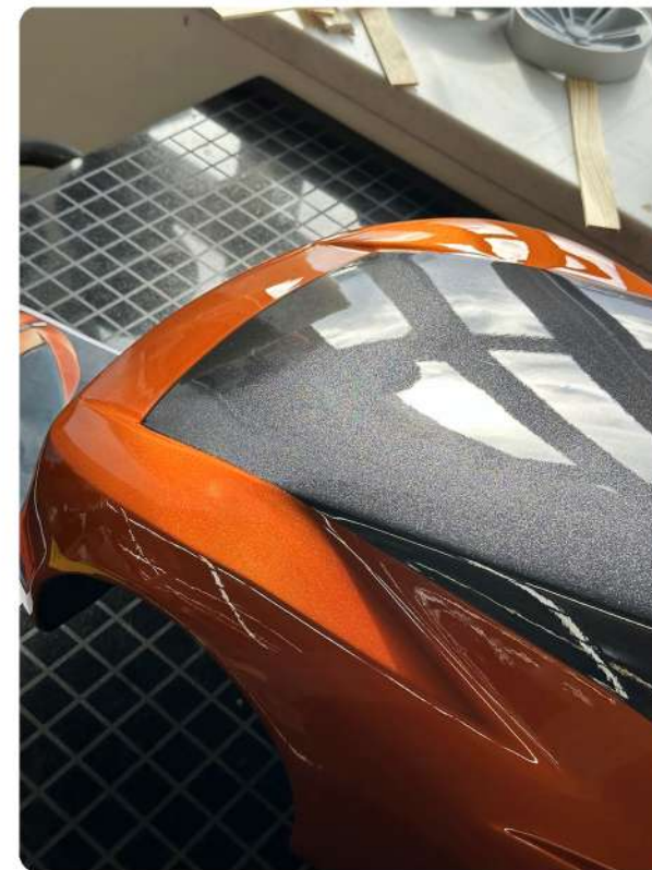
4. Clear Coating and Finishing
